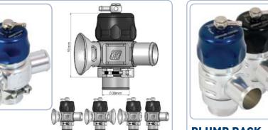
The Dual Port can be configured to vent to the atmosphere, back into the air intake or both! Dual Port is easily the most versatile BOV in the Turbosmart range converting into a Supersonic, Megasonic, (second trumpet supplied for Megasonic mode) Plumb Back or Dual Port. Available in 32mm and 38mm outlet diameters. 19, 25, 29 and 34mm optional plumb back fittings also available.
